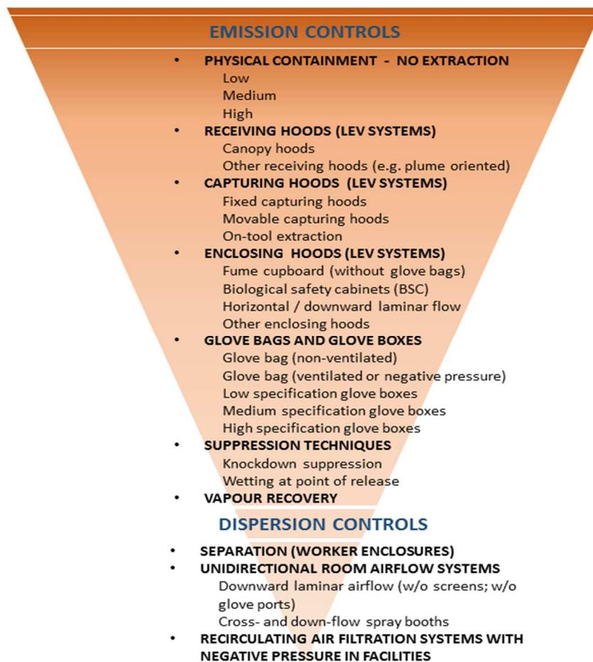
Figure 4. Proposed classification system for engineering controls in air.
