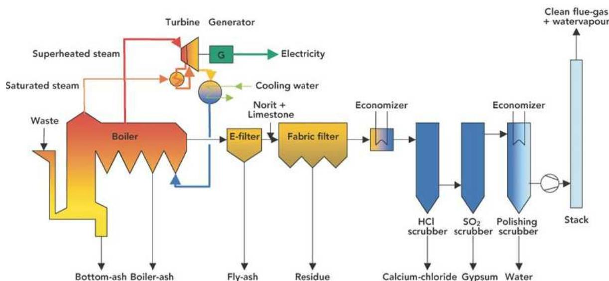
Figure 8. Scheme of waste incineration plant.
