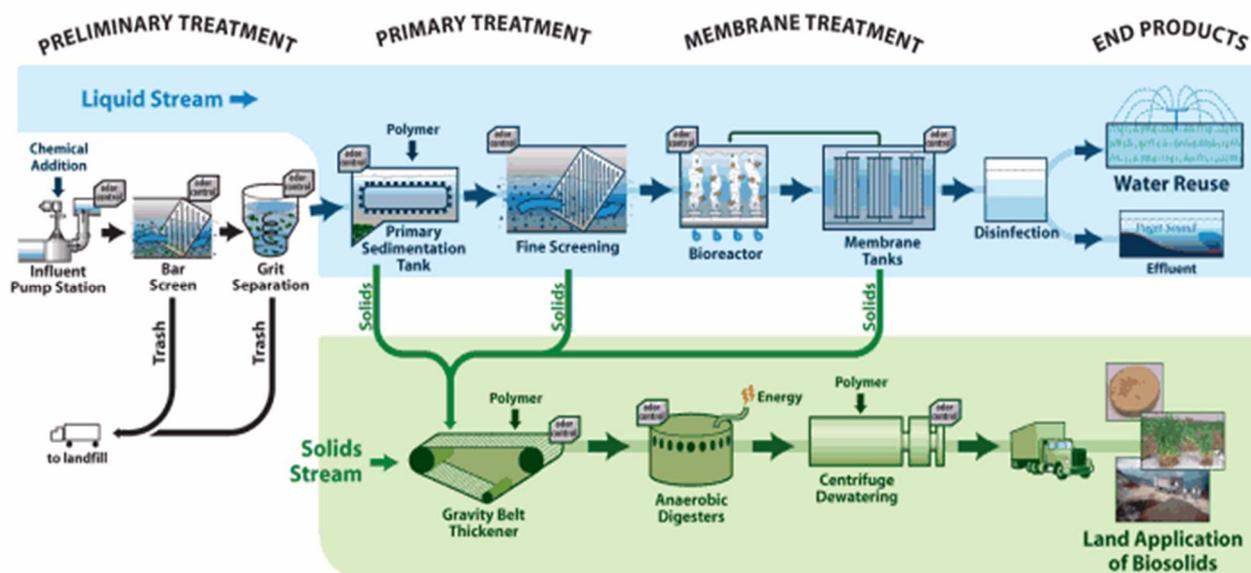
Figure 7. Scheme of water treatment plant.
